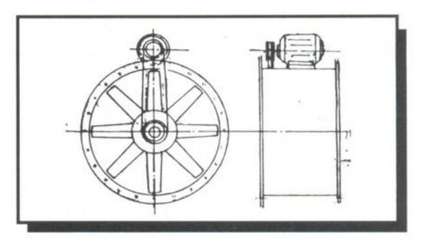
Sweep upto 900 mm. Capacity upto 60000 M³/hr.
