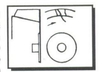
single width single inlet and double width double inlet models. The impeller blades are double curved. These fans find application for ventilation and Air-conditioning.
