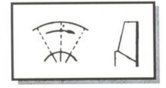
b) Narrow width radial blades for its application in supply air for combustion, forced draft installation, boiler etc.
