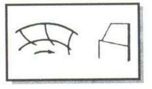
Backward curved redial tip blades making the wheel self-cleaning and are widely used for dust extraction system.
