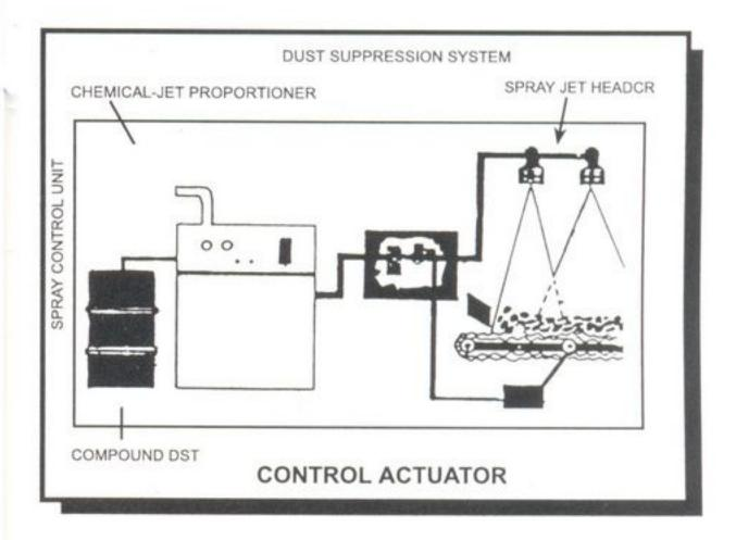
The basic concept of chemical mixed or plain water spray system is to suppress the dust prior to becoming air borne. Generally water mixed with a wetting chemical agent is sprayed in form of fine atomised mist through a proportioner solution pump and spray headers with non-clogging nozzles, forming a shroud and entrapping the dust particles.
