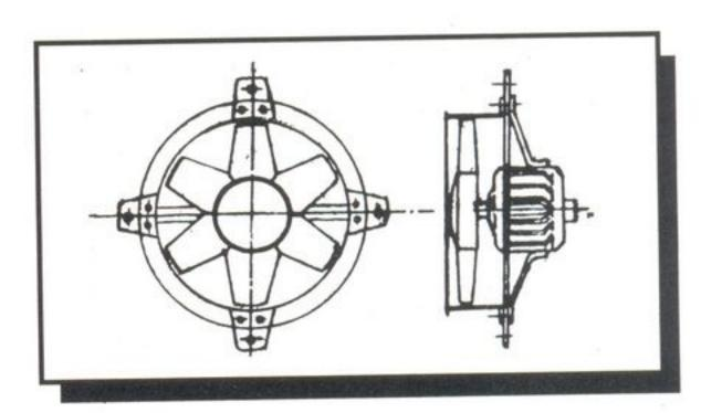
Sweep upto 1200 mm. Capacity upto 90000 M³/hr.
