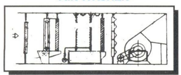
AIR-TECHNIKO Air Washers are designed for the dual purpose of cleaning and cooling of ambient air. The air is passed through self cleaning automatic viscous filter followed by bringing in contact with finely atomised wafer. Due to adiabatic cooling of air the dry bulb temperature tends to reach the wet bulb temperature and thus air is cooled and humidified.
