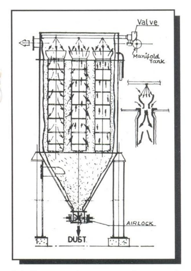
To limit pressure drop across the filter bags, the adjustable solid state timer sequentially opens the solenoid operated diaphragm valves and high energy reverse pulse of clean, oil and moisture free compressed air jet alongwith induced secondary clean air back washes the filter bags.
