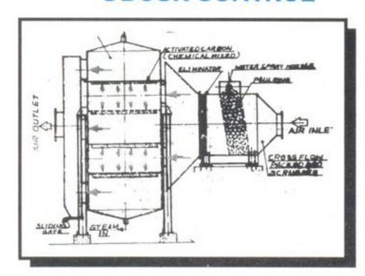
Absorption with chemical treatment and adsorption system.
